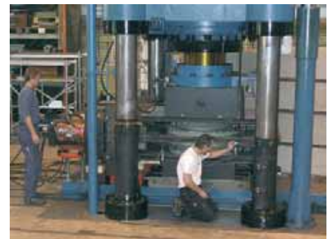
Testing bridge support bearings involves extremely high forces, up to 2000 tonne, applied while simultaneously measuring movements and temperatures.
