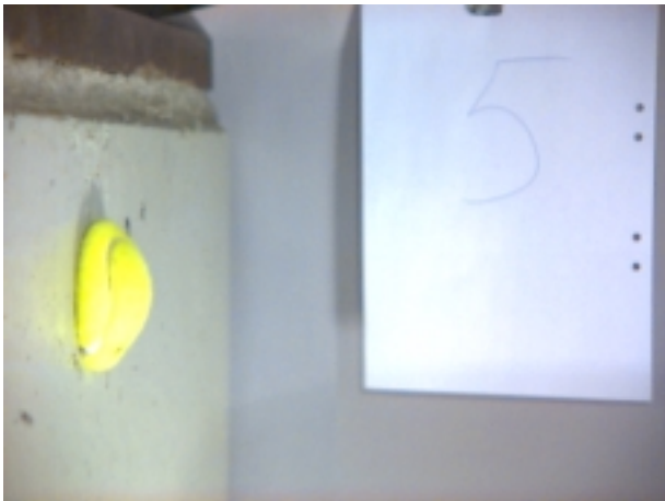
Figure 5: High-speed video showing the maximum deformed state of the tennis ball (velocity=42.4 m/s).
