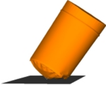
Figure 1: FE-model showing half of the deformed cask (from the inside), dropped from a height of 2m.
