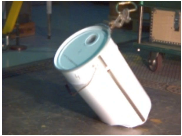
Figure 2: Picture of the impact taken from the video recording, drop height of 2m.
