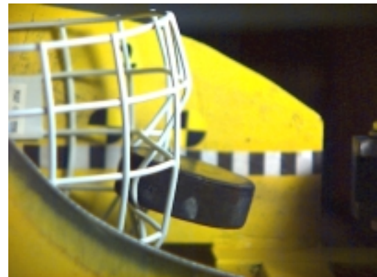
Figure 4: Maximum deformation of the face protector during impact of the puck (velocity=31 m/s) .
