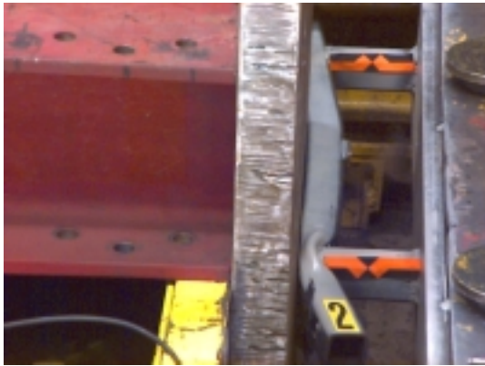
Figure 11: High-speed video recording of the deformation of the bumper during impact.
