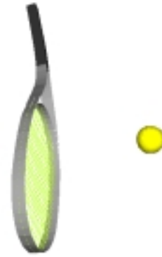
Figure 8: FE-model showing the tennis-ball hitting the strings of the tennis-racket.
