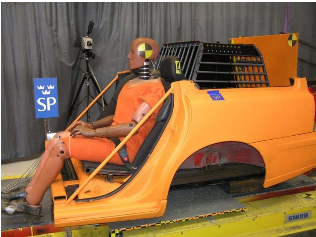
Figure 2, Set-up, rear impact test
