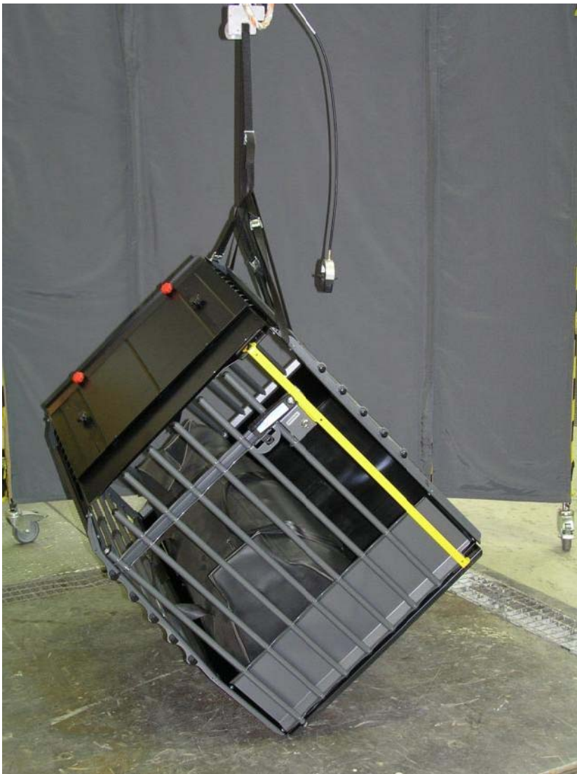
Figure 8, Angle adjustment of the test object before the drop test
