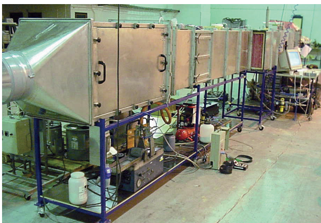
Rig for laboratory tests according to EN 779.
