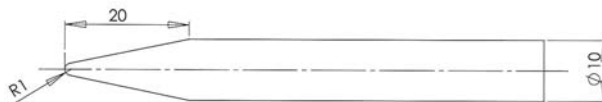
Figure B 2 Pointy probe. Shall be made of metal or other hard smooth material. Measurements in mm.
