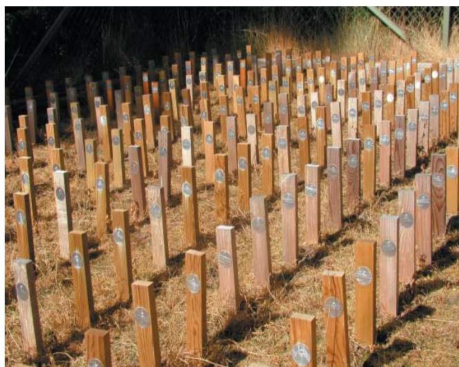
Field test according to EN 252.
