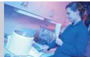
Analysis of grain size distribution in gravel using an air jet sieving.
