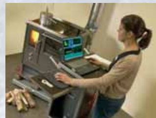
Real-time measurements of particles in small-scale wood-burning are used to gain understanding of transient combustion processes.
