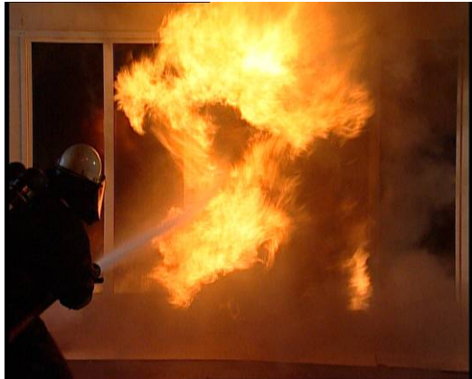
Flashover of a living room
