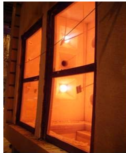
Fire resistance test of a glazing in a fire test furnace
