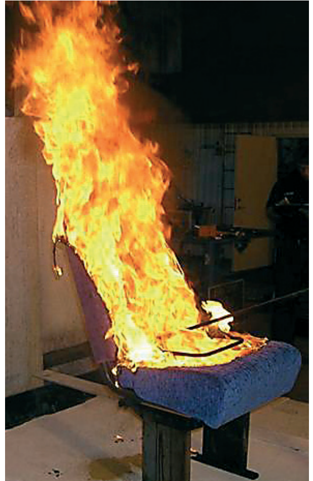
Testing heat release rate from a fire in a seat.
