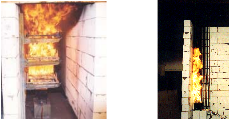
Figure 2 Example of horizontal and vertical real-scale test
