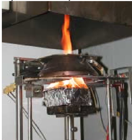
Figure 3 The Cone Calorimeter, a small-scale test method for cables used for modelling cables and for product development
